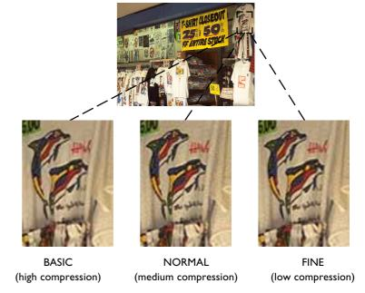
While a setting of NORMAL represents the best trade-off between memory and image quality in most cases, a setting of BASIC can be used to save memory. A setting of FINE is suitable for photographs that will be enlarged or printed at high resolution.
